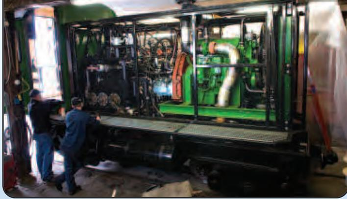
The PowerTech 6125H engine, supplied by Bell Power Systems, features a hospital-grade muffler system to reduce noise. The electronically controlled engine and Funk pump drive power a series of hydraulic components encompassing the powertrain.
