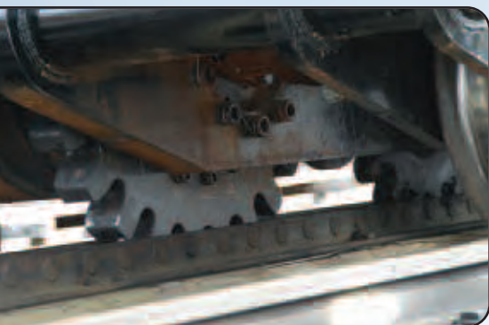
The cog gears beneath the locomotive travel up the tooth-racked rail system.
