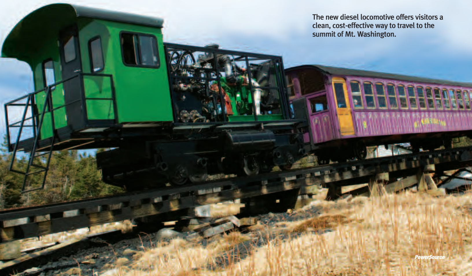
The cog gears beneath the locomotive travel up the tooth-racked rail system.
