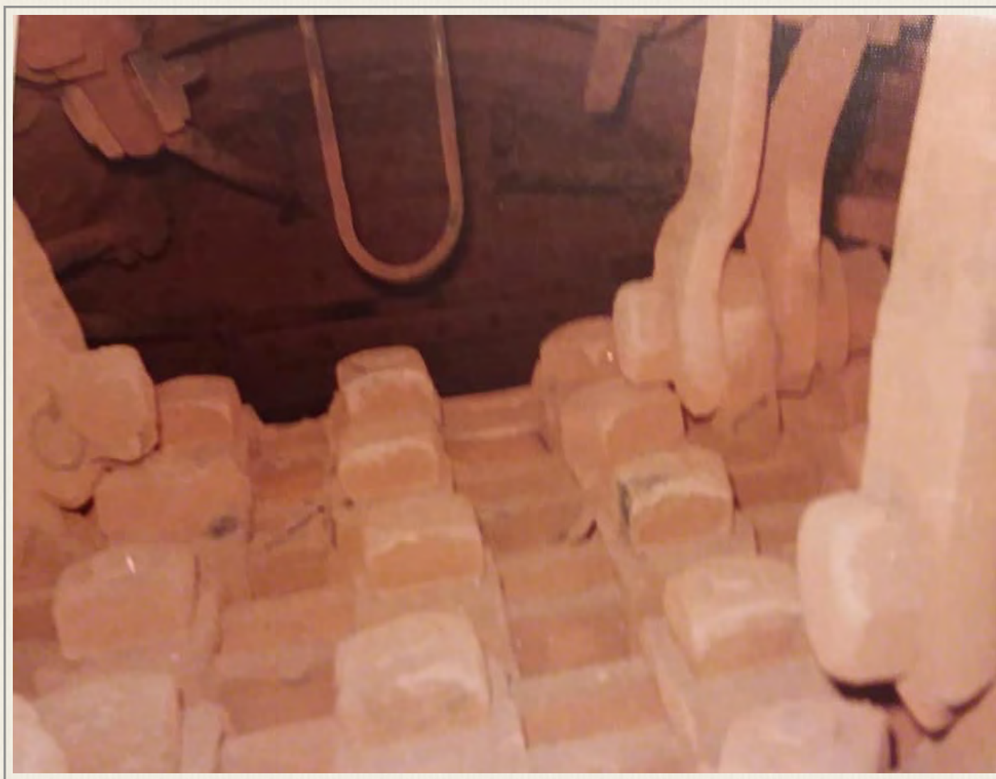
Crown sheet of the #4 - David Huber: "The year I got stuck in the boiler inspecting ferrels on the front flew sheet. Wedged my hips between one of stay rods and top row of flews. Steve Christy had to heat the rod with torch to free me. Ever since this episode, I suffer claustrophobia, which seems to get worse as the years pass." - David Huber photo - MCWR: We Worked There (June 6, 2018)
