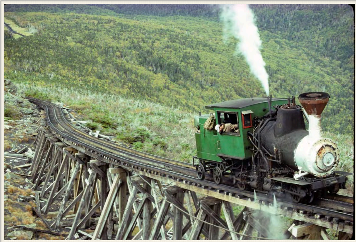
No. 10 became a test bed for the effort to use fuel oil to fire the boiler. Seen here on a test run on Jacob's Ladder (1989) - Rob Bermudes Jr. photo
